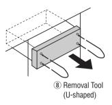
Note: Do not lose Removal Tools. They will be needed to remove the unit from the vehicle's dashboard.
